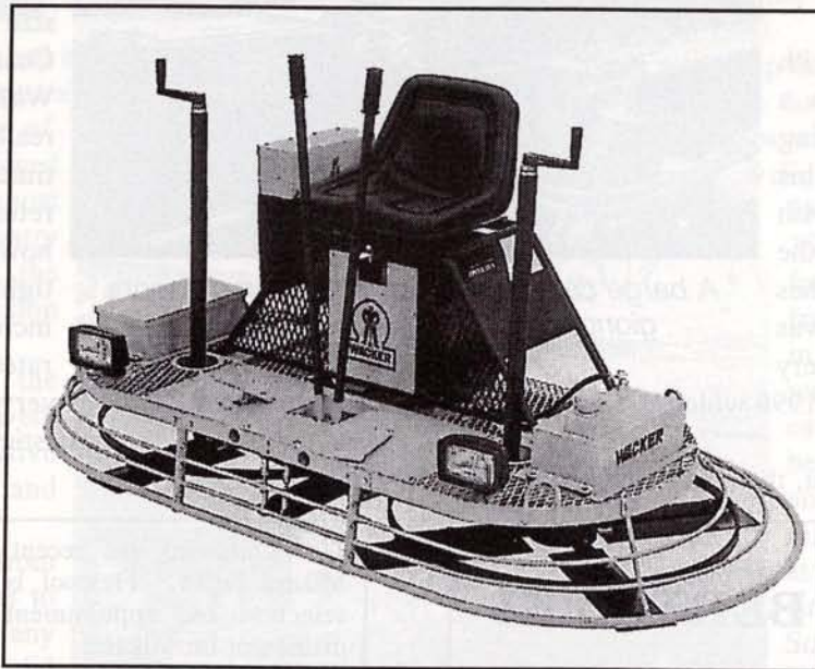
The 46" overlapping ride - on trowel with a Honda engine, CRT 46 ASO, is just one of the four new ride - on trowels added to WACKER's fleet
